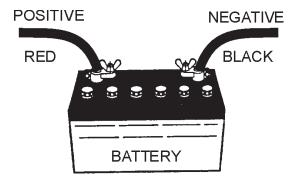
Figure 37. Battery Connections
